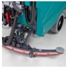
The robust brush deck offers two levels of brush pressure to guarantee excellent cleaning results. Substituting the brushes and pads is easy with the Brush'O-Matic system.
